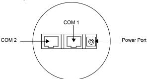
COM 1 connects to the host computer; COM 2 is used for daisy-chaining multiple cradles together; and, the Power Port supplies power to the cradle.
